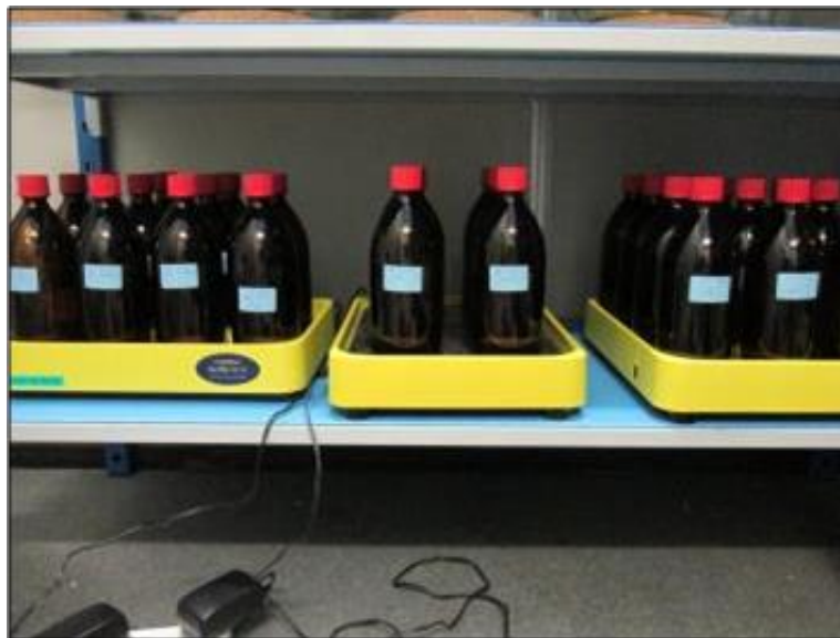
Figure 6. Set-up biodegradation in free water. Simulation of Pelagic zone.
