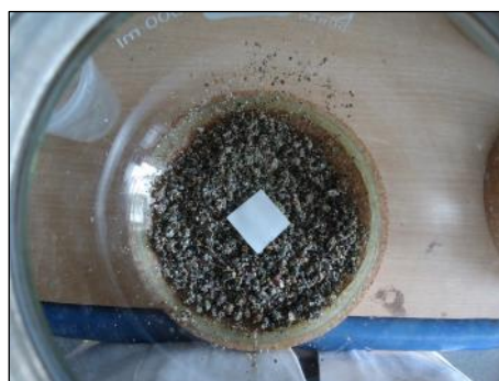
Figure 17. Visual presentation of the specimen (Polyhydroxy alcanoate) on the residual sediment (Greece)
