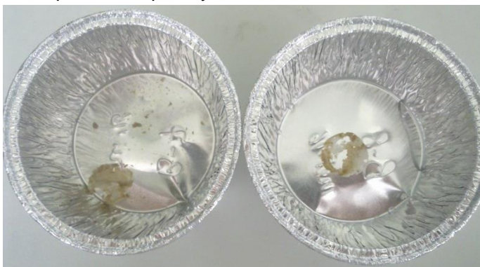
Retrieved PHB test items from (from left to right) BS7, and BS8
