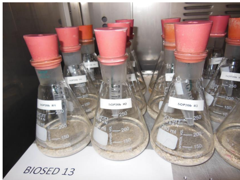
Figure 4. Set-up biodegradation in seawater/sediment interface. Simulation of Benthic zone.
