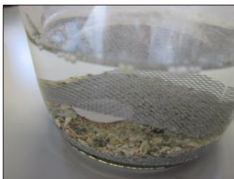
Figure 34. Visual presentation of the use of a mosquito net to prevent floating
