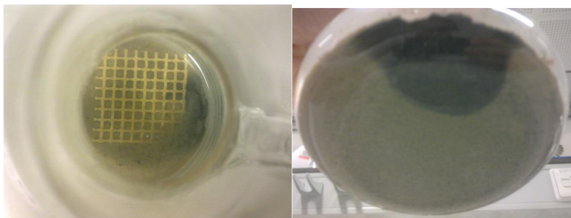
Figure 154. Black staining in bottle BS9 with Greek sediment/seawater and PHB.
