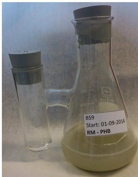
Figure 66. Set up of sandy marine sediment test
