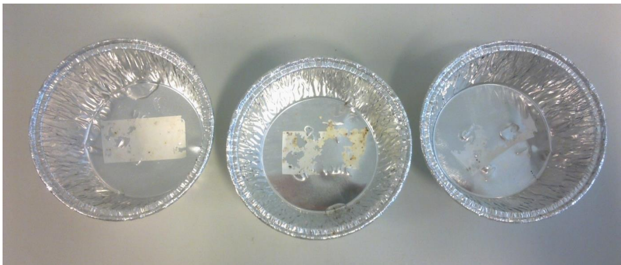
Retrieved PHB test items from (from left to right) T7, T8 and T9
