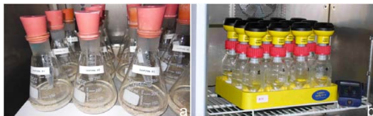
Figure 3. A) Closed bottles of the sublittoral water-sediment interface lab test, measuring the development of CO 2 and b) Oxytop incubation bottles of the pelagic (water column) lab test to measure O 2 consumption.
