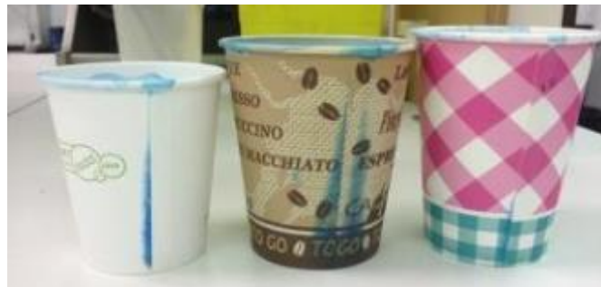
Figure 2 Leakage at the seals for the different coated cups
