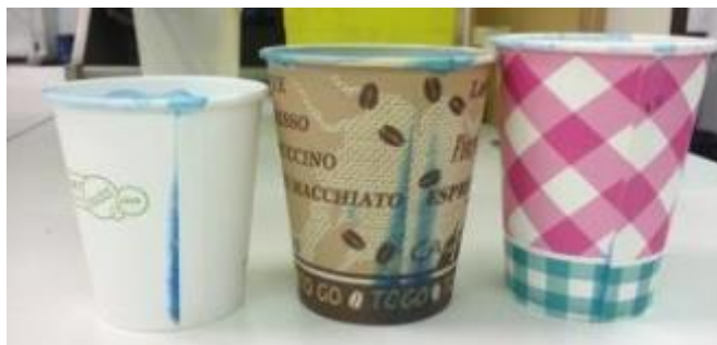
Figure 3 - Leakage at the seals for the different coated cups, from left to right: PLA coated, Ecovio coated and PE coated cups.
